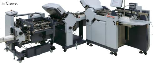
The new machine will be used for folding leaflets accompanying healthcare products for Medica's UK and international clients, including pharmaceuticals giant GlaxoSmithKline. According to IFS, the automated AF-406T6A offers highly flexible processing thanks to its six-by-six buckle-fold configuration, which employs six buckles on the first station and six on the second that can be used in combination.
